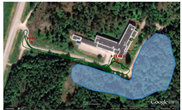
Fig. 2. Aerial photograph of the test field presenting the location of the benchmarks, harvested trees (blue polygon) and the trajectory from the MLS measurements (green dotted curve) (image: Google Earth)
