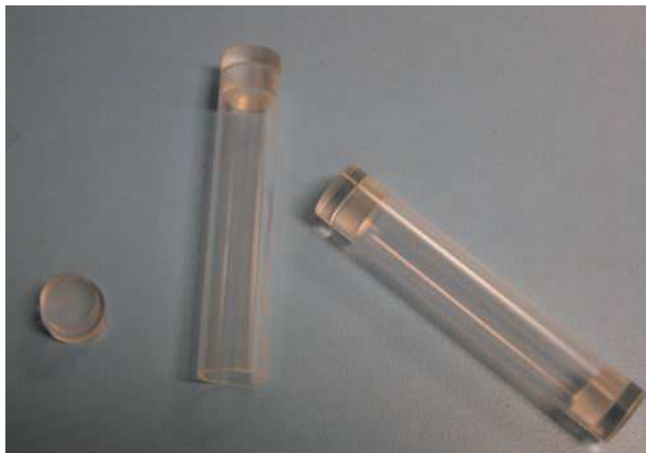
Figure 12: Plexiglas containers for the grease irradiation at 10^{15} 1 MeV n_{eq}/cm^2 .
