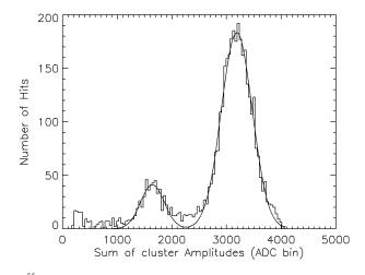
Figure 9: <sup>55</sup>Fe Spectrum acquired with AFTER (200 ns peaking time, 120 fC range).
