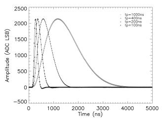
Figure 5: 60 fC test pulses recorded by AFTER with various peaking time (120 fC range).
