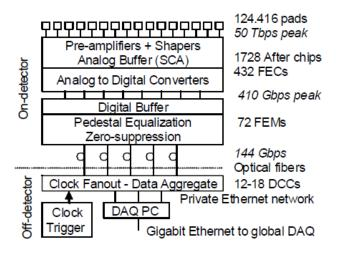
Figure 2: TPC readout flow.
