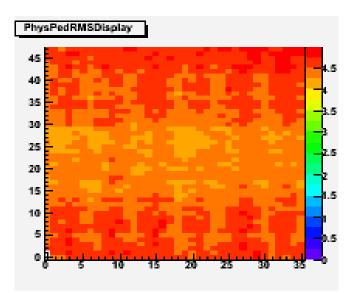
Figure 7: Map of the ENC on a typical Micromégas detector. (120 fC range, 200ns peak time).1 ADC bin corresponds to 164 e-.
