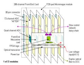
Figure 3: Front-end electronics of one Micromégas module.
