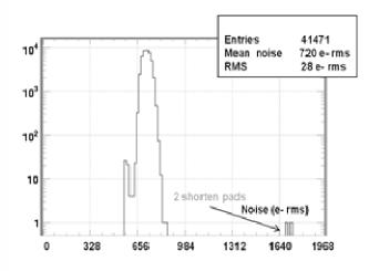
Figure 8: Map of the ENC on a typical Micromégas detector. (120 fC range, 200ns peak time).1 ADC bin corresponds to 164 e-.
