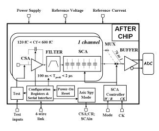
Figure 4: Architecture of the AFTER Chip
