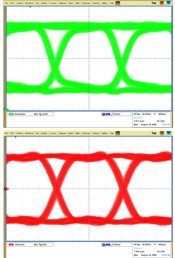
Figure 5: Eye diagram of the near-end transmitter (test point 1, above) and far-end receiver input (test point 4, below) of 5 Gbps, PRBS 2^7-1 data pattern at room temperature.
