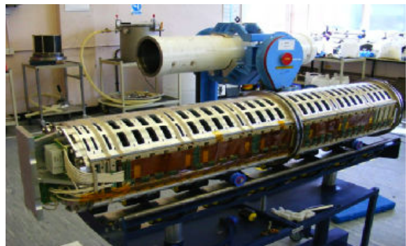
Fig. 9. Medium Voltage Converter: complete assembly.
