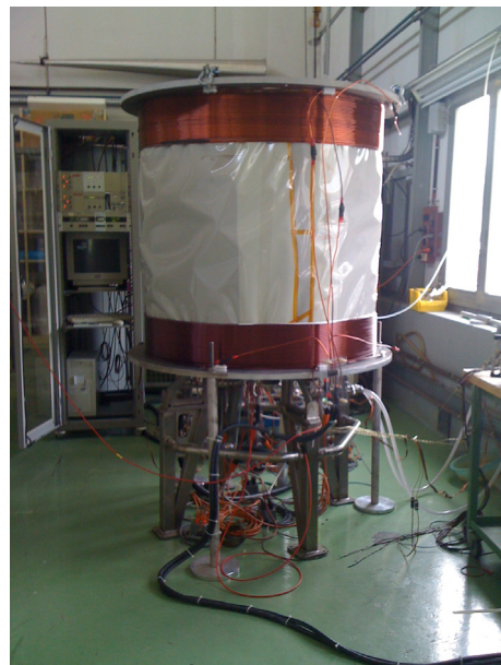
Figure 5: The multilayer coil, 1m diameter, surround the sputtering chamber. Calculations were run to simulate the axial magnetic field and optimize the coil heights.
