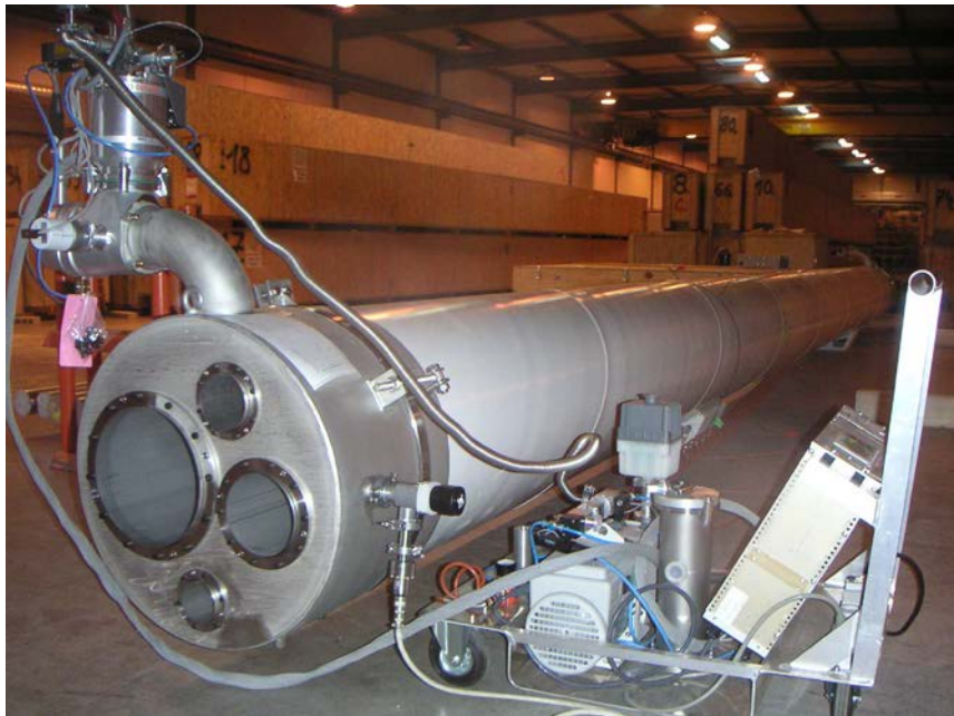
Figure 2 – Stainless steel end dome to close the end of a QRL pipe element
