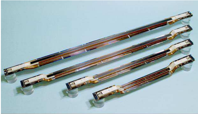
Figure 1: The ladders of all four layers of the present Belle Silicon Vertex Detector (SVD2). In the ladders of the outermost layer, three sensors are ganged and read out by hybrids on either side.
