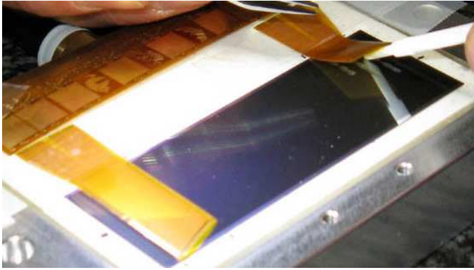
Figure 5: Gluing of the flexes onto the bottom side (long strips) of the DSSD. The pieces are aligned against the bonding pads of the strips and a sample origami hybrid (top left) using a microscope.
