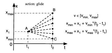
Figure 4-3: Line AB corresponds to the trajectory for control value  $v_{max}$  and line AC corresponds to the trajectory for control value  $v_{min}$ . Triangle ABC is the flow tube used to represent the range of trajectories.
