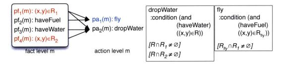
Figure 5-7: The conditions of action dropWater and fly are listed on the right.  $(x, y) \in R_1$  and haveFuel are the resolved conditions of fly.  $(x, y) \in R_1$ ,  $(x, y) \in R_2$  and haveWater are the resolved conditions of dropWater.
