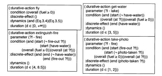
Figure 3-7: In the fire fighting scenario, the air vehicle can perform the following hybrid durative action types: fly, get-water, extinguish-fire, take-photo.
