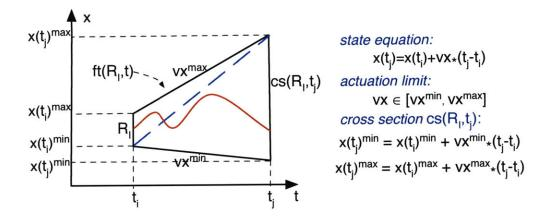
Figure 4-5: Examples of invalid trajectories in a flow tube. There is one state variable, x. There is one control variable, vx. The state equation and actuation limit of the action are listed on the right. Inside flow tube  $ft(R_I, t)$ , two invalid trajectories are shown. The straight dashed line satisfies the state equation, but its control variable value is outside the actuation limit. The curvy solid line satisfies neither the state equation nor the actuation limit.
