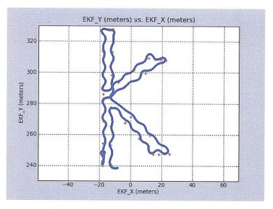
Figure 8-8: The plot of the actual trajectory of Odyssey IV executing the mission script generated by Kongming. AUV's trajectory is in blue dots, and the waypoints planned by Kongming are in red crosses.
