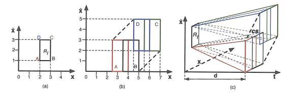
Figure 1-7: An example of a flow tube of a hybrid action in 1D for a second-order acceleration limited dynamical system. (a) shows the initial region  $R_I$ . (b) shows the end region. (c) shows the flow tube of duration d.
