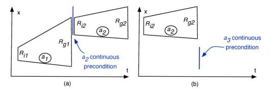
Figure 1-8: (a) Flow tube  $a_2$  is connected to flow tube  $a_1$  because the end region of  $a_1$  has a nonempty intersection with the continuous condition of  $a_2$ . (b) Conversely, flow tube  $a_3$  is not connected to flow tube  $a_2$  because the end region of  $a_2$  has an empty intersection with the continuous condition of  $a_3$ .
