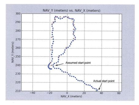
Figure 8-5: The plot of the actual trajectory of Odyssey IV executing the mission script generated by Kongming. AUV's trajectory is in blue dots, and the waypoints planned by Kongming are in red crosses. The extra leg close to the bottom of the plot occurs because at the start of the mission, the vehicle was not at the assumed start location. Hence it had to traverse to the assumed start location first.
