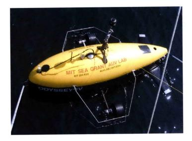
Figure 8-1: Odyssey IV, an AUV from the MIT AUV Lab at Sea Grant, is  $0.7 \times 1.4 \times 2.2$ m, weighs 500kg dry and about 1000kg wet, and has rated depth 6000m. More information about the vehicle can be found in [ody].
