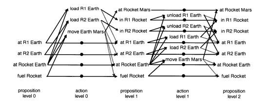
Figure 4-7: A Planning Graph of 3 proposition levels and 2 action levels. Round black dots represent no-op actions. Solid lines connect conditions with actions and actions with add-effects. Dotted lines connect actions with delete-effects.
