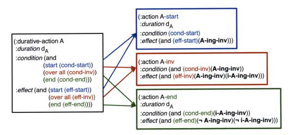
Figure 6-2: The LPGP encoding of a durative action. On the left-hand side of the figure, there is the specification of a durative action A. On the right-hand side of the figure, there is the specification of the *start* action, the *inv* action, and the *end* action.
