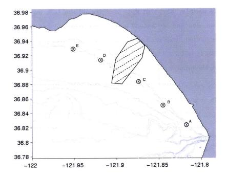
Figure 1-1: Map for the sampling mission in Monterey Bay. Grey area is land, and white area is ocean. Engineers characterize the area with traffic and fishing activities with a shaded polygon in the map. It is the obstacle that the AUV needs to avoid. *Picture courtesy of MBARI.*
