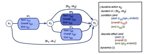
Figure 1-12: Hybrid durative action type  $a_2$  is created for goal episode  $ge_2$ .  $ge_1$ -ended and  $ge_2$ -ended are literals, representing respectively the fact that  $ge_1$  and  $ge_2$  are achieved.  $c_{s2}$ ,  $c_{i2}$  and  $c_{e2}$  are the constraints at different times of  $ge_2$ .
