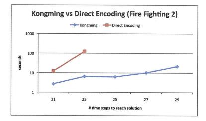
Figure 8-13: Logarithmic scale plot of the result of Fire-fighting Scenario 2. The horizontal axis is the number of time steps to reach solution. The vertical axis is computation time in seconds. Blue line shows the performance of Kongming. Red line shows the performance of Planner<sub>DE</sub>. Kongming scales well. However, after time step 23, the computation time of Planner<sub>DE</sub> goes beyond 48 hours.
