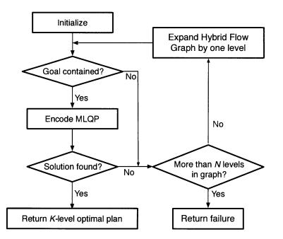
Figure 5-3: The algorithm for  $K_{AA}$ .
