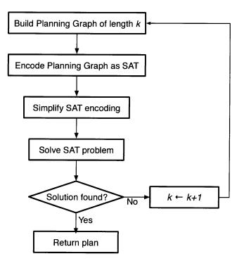
Figure 5-1: The algorithm architecture of Blackbox.
