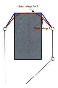
Figure 8-2: Comparison of an example of a corner-cutting path with a VG-preprocessed path. The blue path shows the path when using the VG pre-processing, and the red path shows the path without the VG pre-processing. As we can see, along the red path, the position at time step i and the position at time step i + 1 are outside the obstacle, but the path in between the two time steps is undesirably inside the obstacle.
