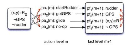
Figure 5-8: startRudder and glide are mutex actions. getGPS and no-op are mutex actions. rudder and  $(x, y) \in R_1$  are mutex facts. GPS and  $\neg$ GPS are mutex facts.
