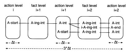
Figure 6-6: Action A-end is in action level i + 2, its matching A-start action is in action level *i*. If A-end takes place, then the time between the beginning of action level *i* and the end of action level i + 2,  $3 * \Delta t$ , needs to be within the duration bounds on A's duration.
