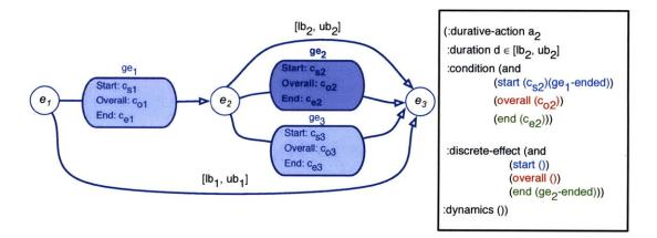
Figure 7-3: Hybrid durative action type  $a_2$  is created for goal episode  $ge_2$ .  $ge_1$ -ended and  $ge_2$ -ended are literals, representing respectively the fact that  $ge_1$  and  $ge_2$  are achieved.  $c_{s2}$ ,  $c_{o2}$  and  $c_{e2}$  are the constraints at different times of  $ge_2$ .
