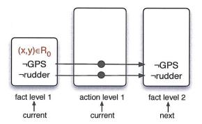
Figure 4-22: No-op actions are created for literal  $\neg$ rudder and literal  $\neg$ GPS in fact level 1, represented by black dots.
