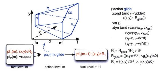
Figure 5-10: Action glide in action level m. Its type definition is listed on the right.  $R_{glide}$  is its continuous condition, specified by a conjunction of linear inequalities.  $R_0$  is its resolved condition in fact level m, also specified by a conjunction of linear inequalities.
