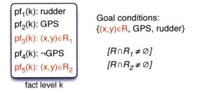
Figure 5-5: An example of the last level of a k-level Hybrid Flow Graph. The goal conditions are listed on the right.
