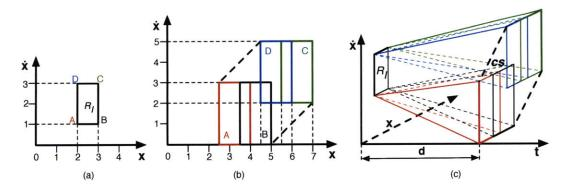
Figure 4-4: An example of constructing a flow tube of an action in 1D for a secondorder acceleration limited dynamical system. (a) shows the initial region  $R_I$ . (b) shows the cross section of  $R_I$ . (c) shows the flow tube of duration d.
