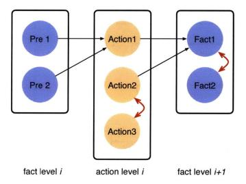
Figure 5-2: A Planning Graph example to demonstrate the encoding rules of Blackbox. "Pre1" and "Pre2" are conditions of "Action1". "Action1" and "Action2" both have "Fact1" as an effect. "Action2" and "Aciton3" are mutex. "Fact1" and "Fact2" are mutex.
