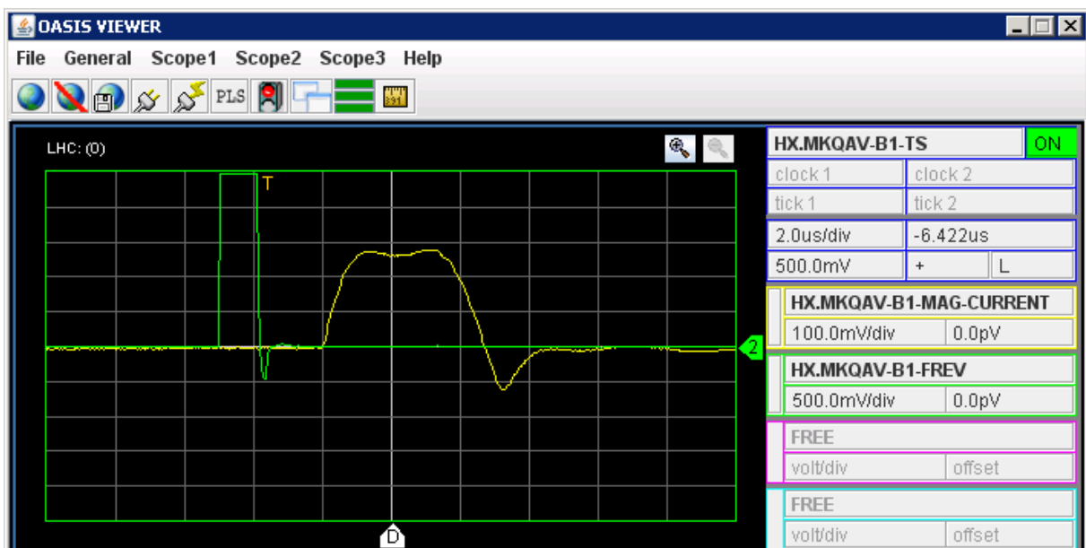
Figure 23 OASIS remote viewing window depicting 'Q' mode magnet pulse response
