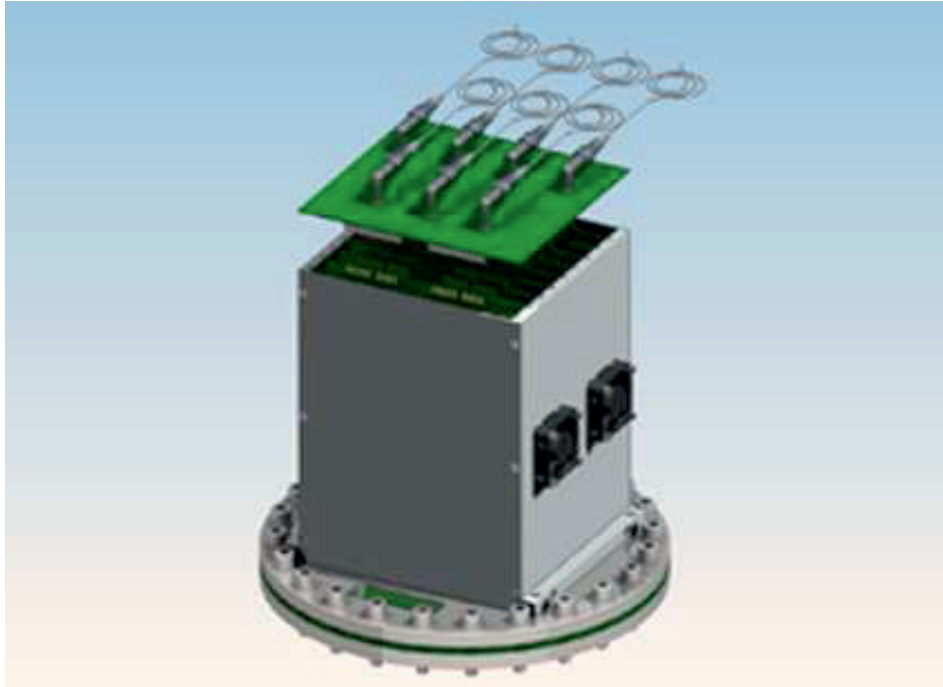
Fig. 6: Artistic view of ICARUS DAQ mounted on the flange with serial ADCs and optical link.
