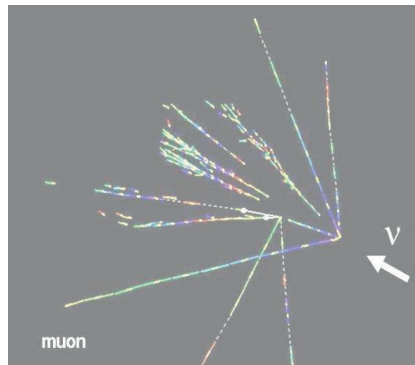
Fig. 2: A neutrino interaction reconstructed in ECC with a secondary hadron interaction. Six electromagnetic showers have been reconstructed in the event: four of them from the primary and two from a secondary vertex.
