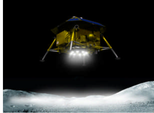
(b) Equatorial variant of JAXA's proposed SELENE-2 lander
