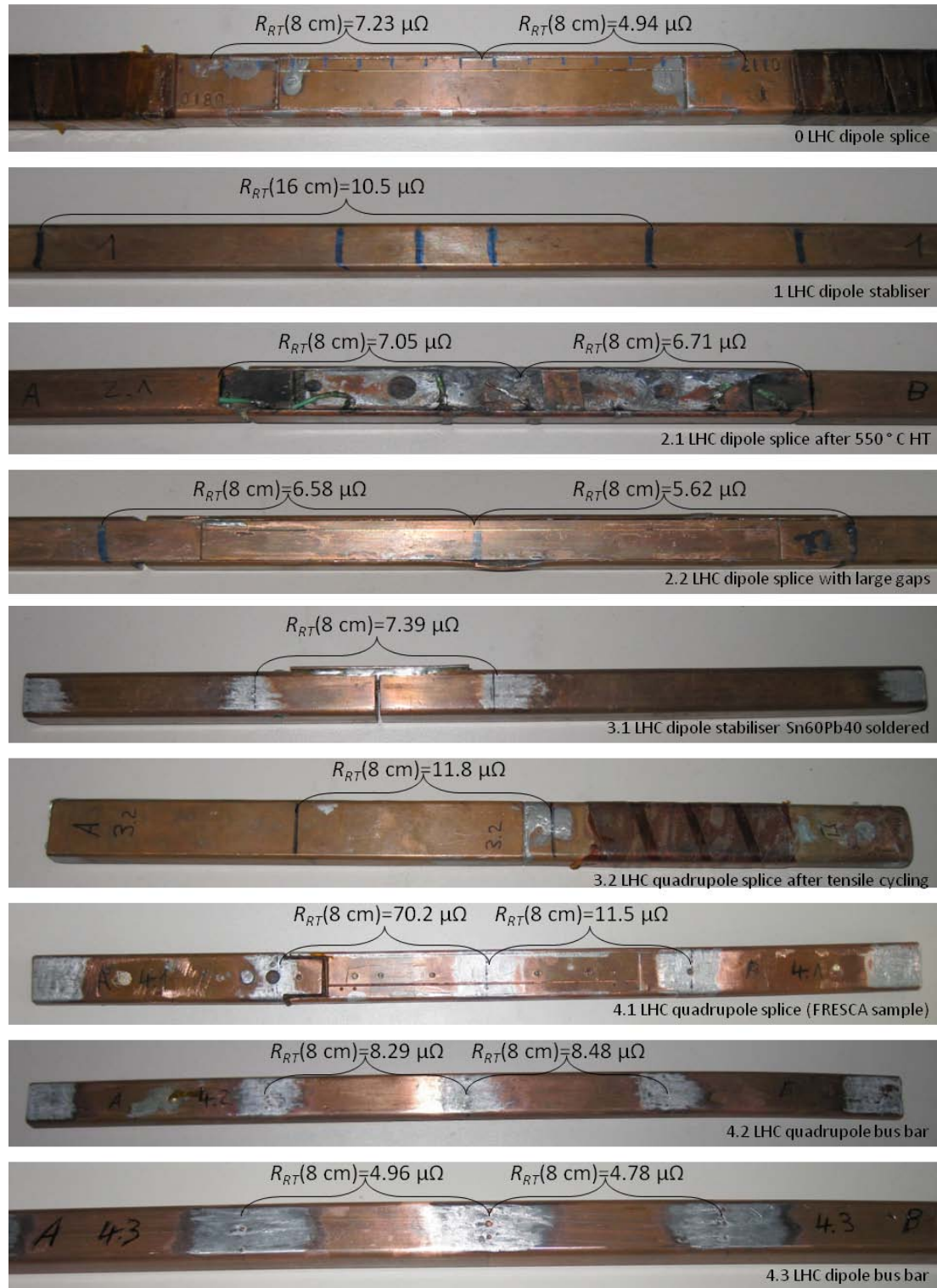
Figure 3: Different samples used for resistance measurements. The voltage tap positions and the RT resistance results are indicated for all samples.
