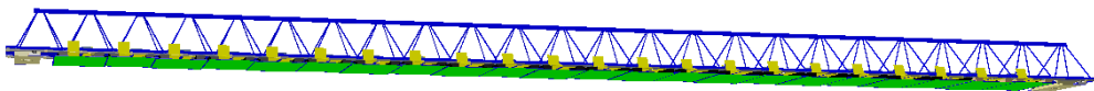
Figure 5: View of one SSD ladder (from layer 5) as described in the AliRoot geometry.
