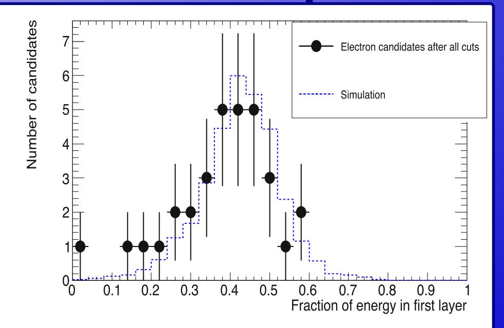
Typical shower shape variable for electrons - the fraction of total energy left in first layer of electromagnetic calorimeter. Distribution of final ionisation electrons compared to Monte
