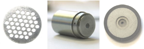
FIG. 4. The modified pieces for the two prototypes: accelerating grid (left), anode body (center) and outlet plates (right).
