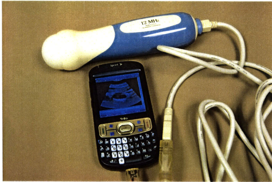
Figure 43 Interson probe with a Windows Mobile Palm Treo 800w running Cell Phone SDK (74)
