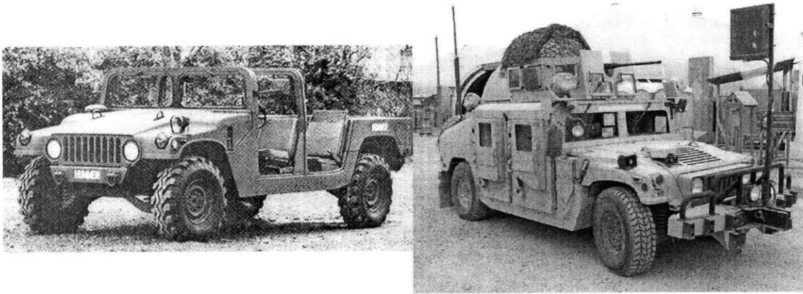
Figure 1-4: Evolution of HMMWV, from 7500 lb GVW prototype (Dunne, 1982) to 17,900 lb armored vehicle (Anderson, 2009)
