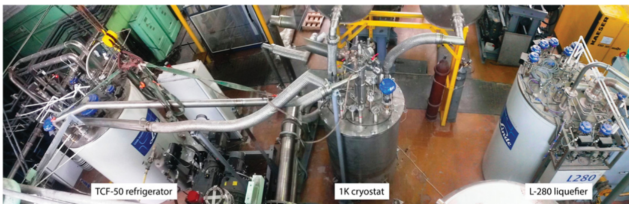
Figure 4. Photograph of the full-scale model of the UCN source for the WWR-M reactor.
