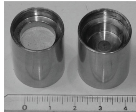
Figure 8. First prototypes of a superleak filter. They employ compressed \text{Al}_2\text{O}_3 powder with grain sizes 100 nm and 25 nm, respectively.
