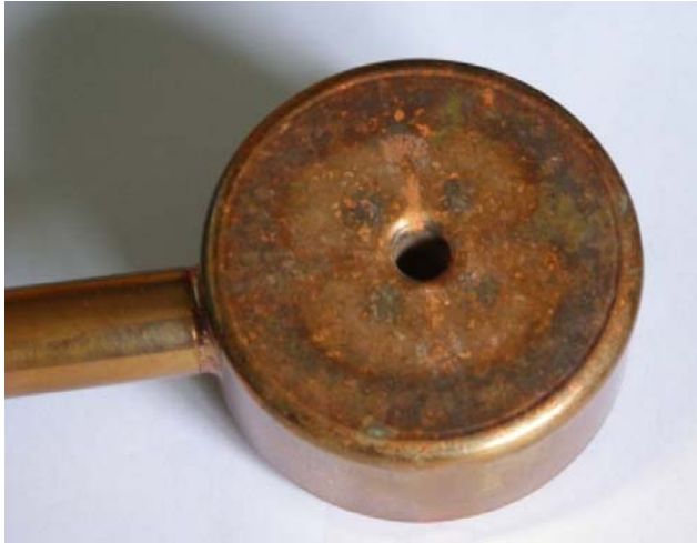
Figure 5. 425 MHz drift tube showing the PMQ fringe-field pattern.
