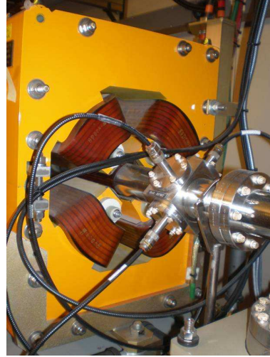
Fig. 23: Scheme of a rotated button BPM arrangement (left) and a photo of the realization mounted close to a quadrupole magnet at the ALS Booster-synchrotron, Berkeley (right)
