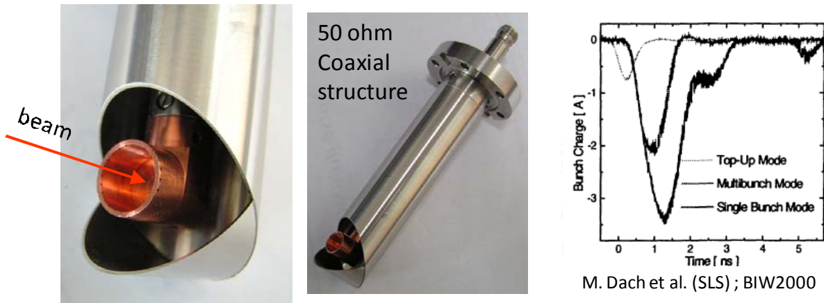
Fig. 5: A wide-bandwidth retractable Faraday cup built at SLS
