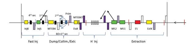
Figure 1: Long straight section layout, including collimators, injection and extraction elements.
