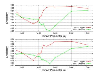
Figure 2: Global efficency for different impact parameters with collimators in LSS1 (bottom) and in LSS2 (top).
