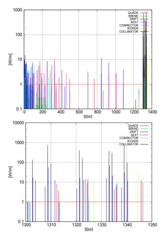
Figure 3: Beam loss maps when collimators are placed in LSS1 (top) and zoom around the collimator section (bottom).
