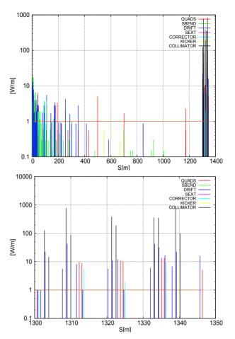
Figure 4: Beam loss maps when collimators are placed in LSS2 (top) and zoom around the collimator section (bottom).
