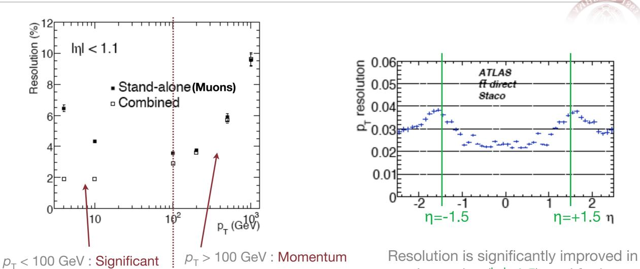
Muon spectrometer crucial for good momentum resolution at large pT.
