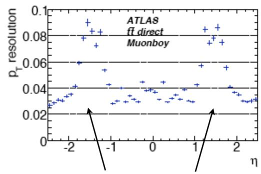
Resolution is degraded in the region  $1.2 < |\eta| < 1.7$  mainly due to the low field integral , but also the limited number of measurements, and the large amount of material
