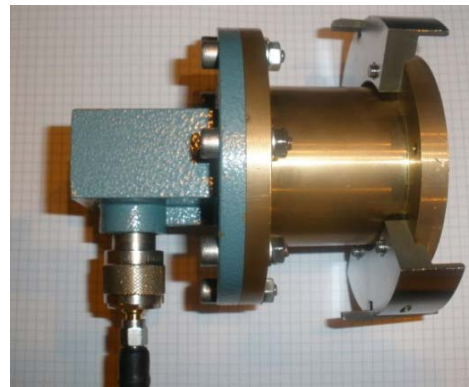
Figure 4.10 Picture of TE-mode coupler[10]
