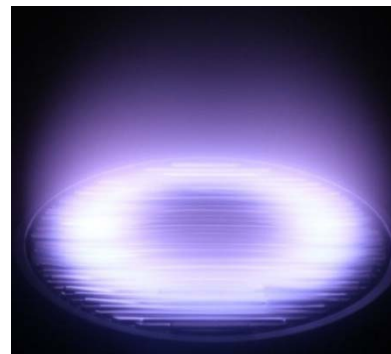
Figure 3.6 Plasma over magnetron[10]
