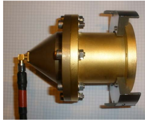
Figure 4.8 Picture of TM-mode coupler[10]
