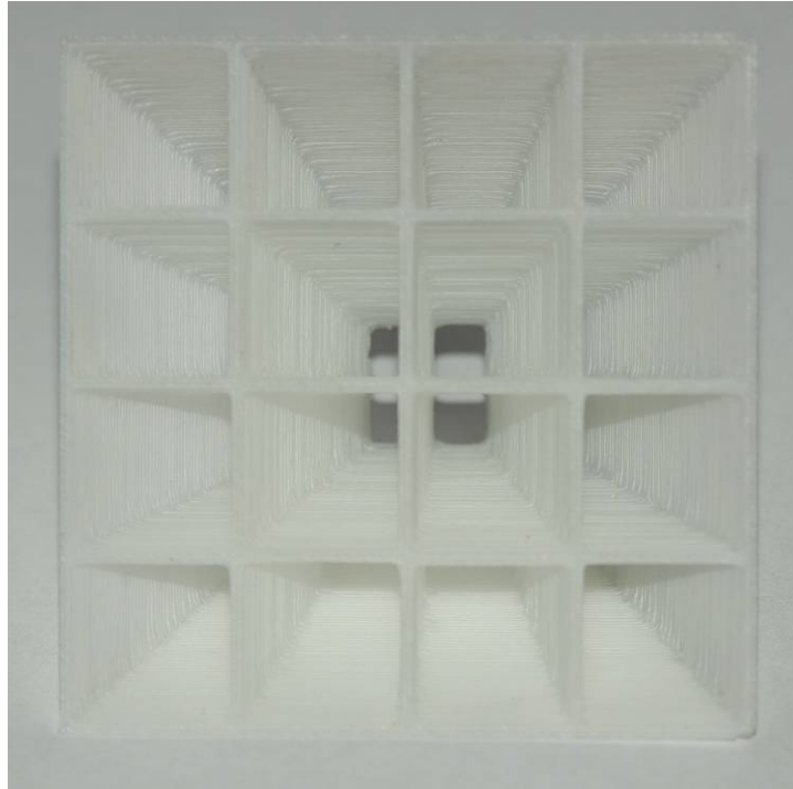
Figure 3.7: Photo of the plastic prototype of a hollow waveguide. The system length was cca 30mm. The fine structure is caused by the rapid prototyping method.
