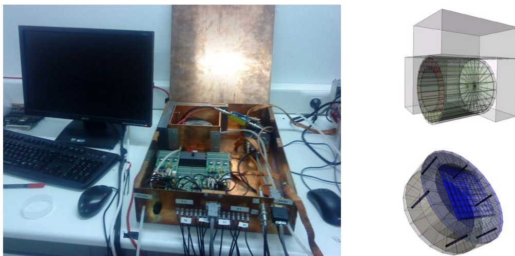
Figure 19. Left: CAST based acquisition system with a dedicated Faraday cage prepared for the low background measurement tests. Detector M13 is actually installed in the Faraday Cage. The copper cage is specially designed to fulfill a minimum leak rate to flush the detector with Nitrogen. Right: Parts of the micromegas simulation, shielding and detector.
