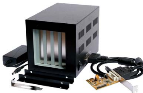
Figure 4. New PCI Box Extension connected to the Slow Control PC.
