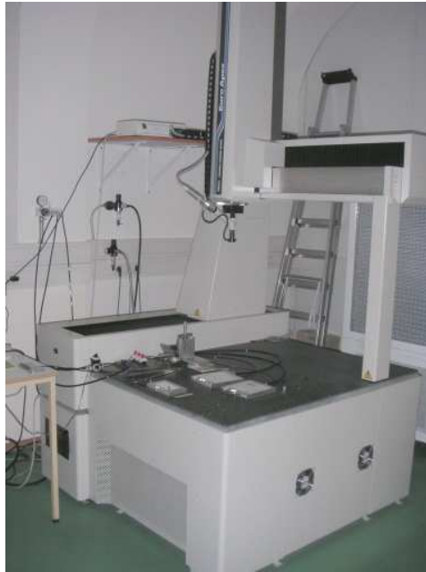
Figure 42: The coordinate measuring machine used to ensure proper alignment of the individual components on the module.
