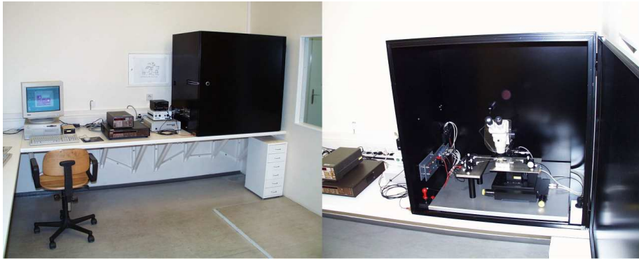
Figure 31: Pictures of the probe station setup. The left picture shows a long shot of the equipment including the computer, the measuring devices and the light tight box. The right picture shows a closer look into the box. A microscope, the contact needles and the motorized XY-table can be seen.
