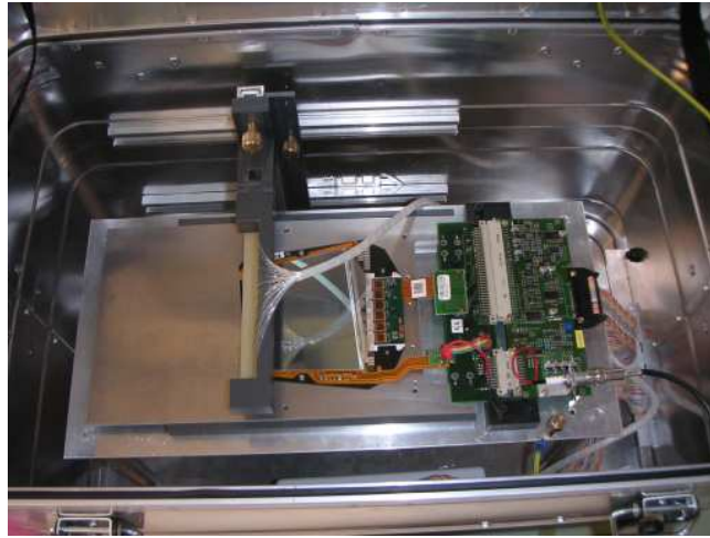
Figure 48: The inside of the test box. The LED emitter is placed just over the sensor and on the left the FE adapter can be seen.
