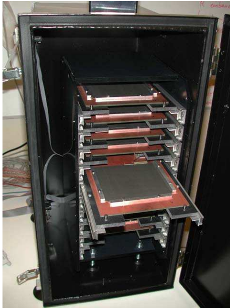
Figure 36: The opened Sensor Box. One of the tables is extended and the conductive rubber which connects the bias voltage to the backplane can be seen.
