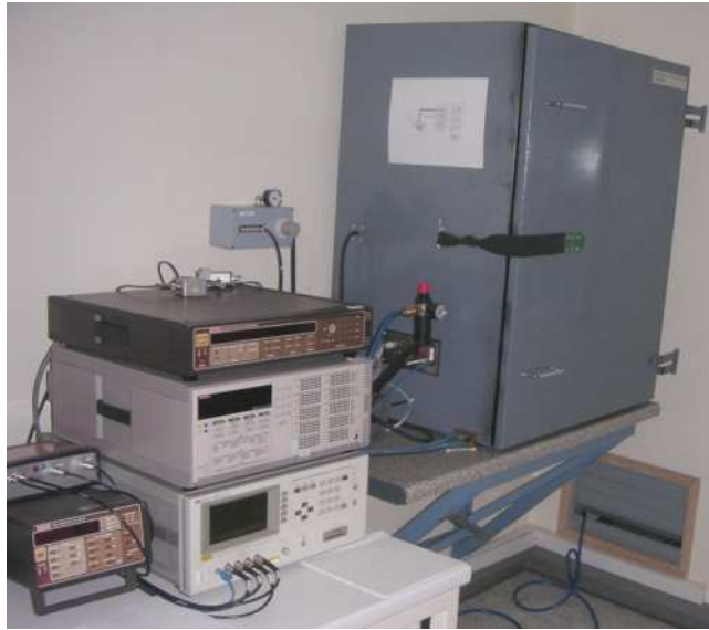
Figure 40: The PQC setup. On the left side the necessary electronics can be seen and on the right side is the gray light tight box
