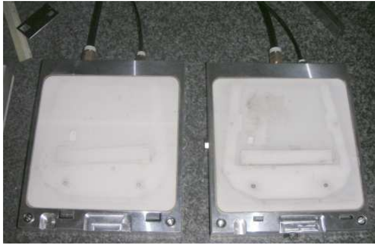
Figure 41: The chucks used for placing the components during assembly. The recess for the components can be weakly seen.
