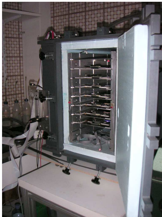
Figure 49: The cooling box loaded with several modules. The thick isolating material can be clearly seen on the door and inside the box.
