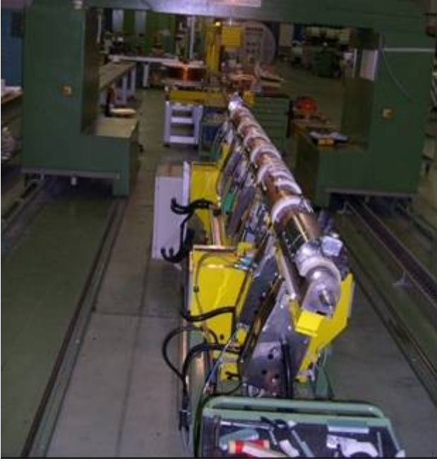
Fig. 2: Winding operation with a dummy conductor. The geometrical curvature is clearly appreciable.
