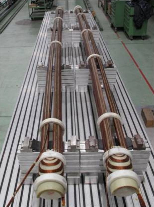
Fig.3: Two complete poles, after curing,
