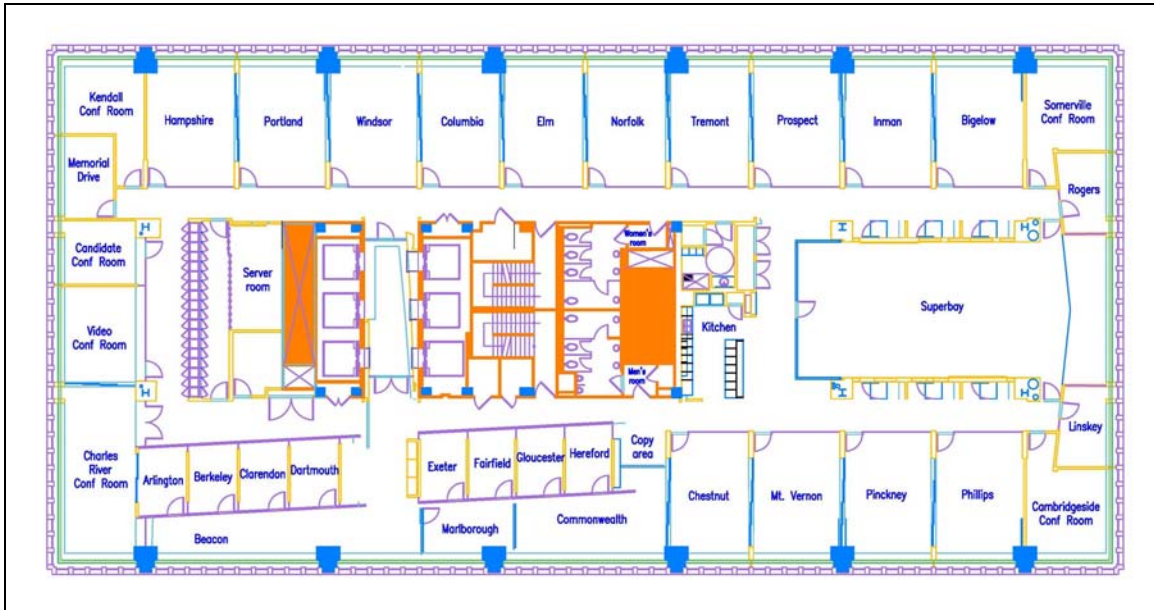
Figure 3.11: Plan of Cambridge Innovation Center: Company bays with movable walls allow for seamless growth. Meeting rooms occupy the corners for the best view and maximum prestige. A superbay serves hot-desk workers. Source: Cambridge Innovation Center
