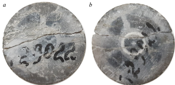
Fig.3. Images of the ends of the core sample from the side of the well (a) and from the side of the reservoir (b) with a natural fracture
