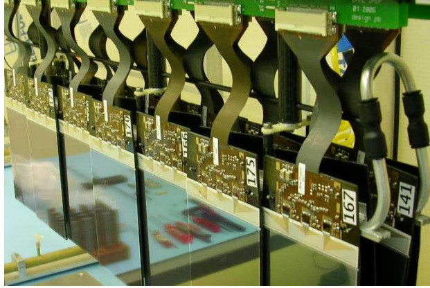
Figure 19: Photo of the IT layers fixed to the aluminium cooling rod. Both the X and stereo layers are visible, as well as the cooling-rod bending on the right of the picture.
