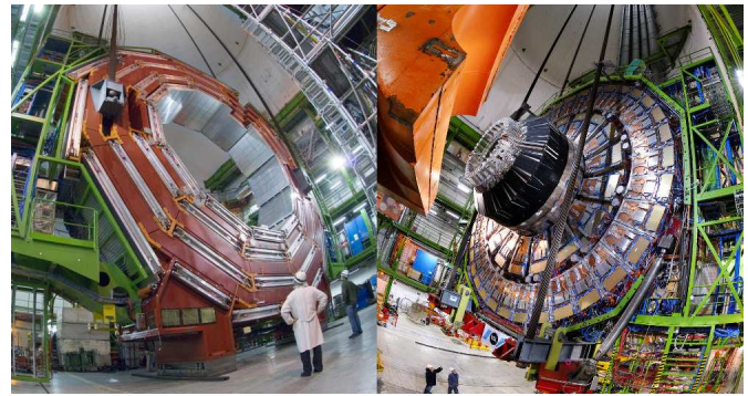
Figure 2: Lowering of CMS slices, a barrel wheel (left) and one of the endcap disks (right).
