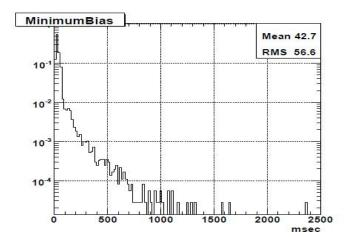
**Figure 5**. Timing profile for the HLT menu developed for LHC luminosity  $L = 1032 \,\mathrm{cm}^{-2} \mathrm{s}^{-1}$  for a sample of QCD events passing the L1T selection. The results are obtained on a PC mounting 3 GHz Intel CPU [16].
