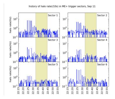
**Figure 11**. Muon halo rates recorded in the muon end-cap (ME) trigger sectors, at the passage of the beam through CMS. The yellow band shows the beam capture signal recorded downstream of the CMS detector.
