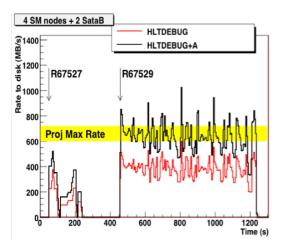
**Figure 9.** Rate of data to disk as a function of time for two cosmic rays runs where the high rate randomly triggered events were only partially filtered out by the HLT, thus saturating the bandwidth of the storage system. The contributions from the two data streams implemented during those runs are shown separately.
