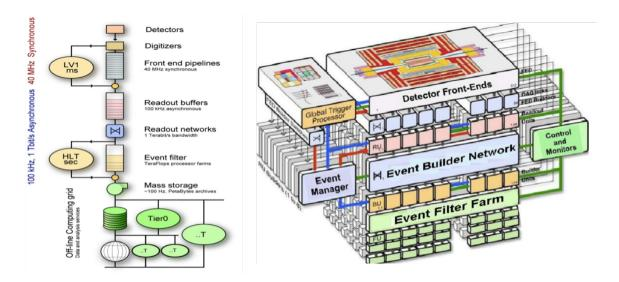
**Figure 1**. Left: schematic view of the CMS Trigger and DAQ architecture. Right: representation of the DAQ system from the front ends to the storage system. The development in the third coordinate corresponds to the implementation of several independent DAQ slices.
