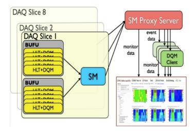
Figure 4. Schematic representation of the monitoring data flow.
