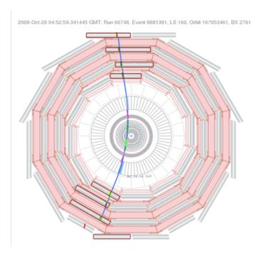
**Figure 8**. Event display of a cosmic muon reconstructed online in the HLT. Information from the muon chambers, calorimeters (m.i.p energy deposits) and tracking system are used to fit the muon track throughout the full detector.
