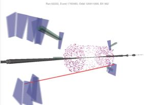
nated from  $(2 \times 109)$  protons hitting the collima- a beam halo muon. tor blocks situated about 150 m upstream of CMS, were detected in the calorimeters (calorimeter deposits shown in blue) and muon chambers (muon chamber hits shown in green).
