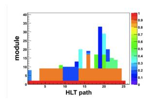
**Figure 10**. Example of DQM histogram for the monitoring of the HLT performances. The HLT paths are listed on the horizontal axis, whereas the vertical axis represents the depth along the reconstruction sequence. The color code expresses the rate at which a given reconstruction module is executed. This result is for a cosmic muon run with dedicated HLT menu.
