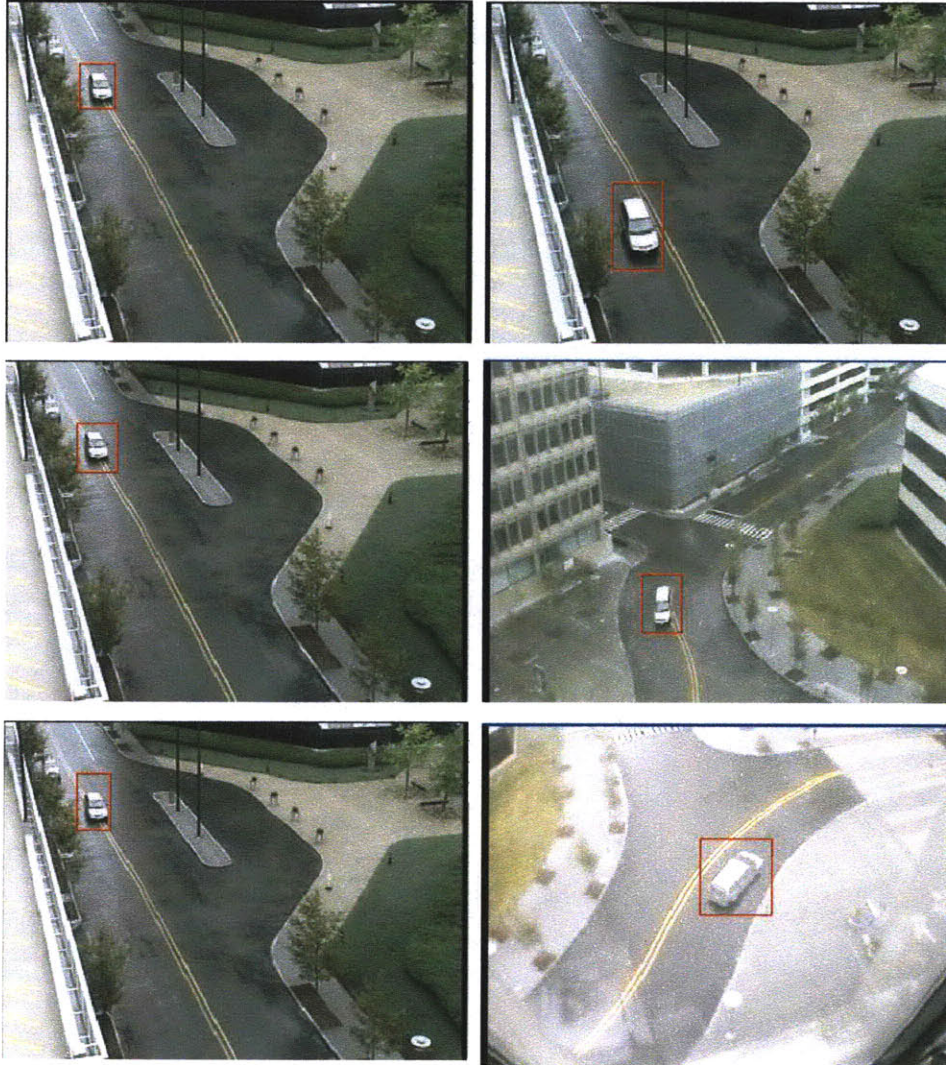
Figure 1-2: Tracking examples. The bounding box shows the moving object. The first row shows tracking through the same view, the middle row shows tracking through overlapping camera views, and the bottom row shows tracking through non-overlapping camera views.
