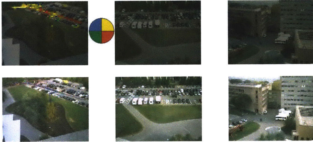
Figure 4-6: Learned cluster 3: the first row shows the learned activity cluster 3 and the second row shows the trajectories clustered into this activity. This cluster captures vehicles entering the parking lot and parking immediately without appearing at Camera 2.
