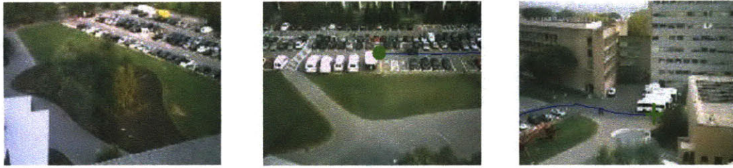
Figure 4-9: Abnormal activity 1: A vehicle left Camera 3, entered Camera 2 with the wrong moving direction and then stopped. In this case, the moving direction in the Camera 2 is unusual. The trajectories is plotted in blue, and the starting and ending points of the trajectory are marked by green plus and dot.
