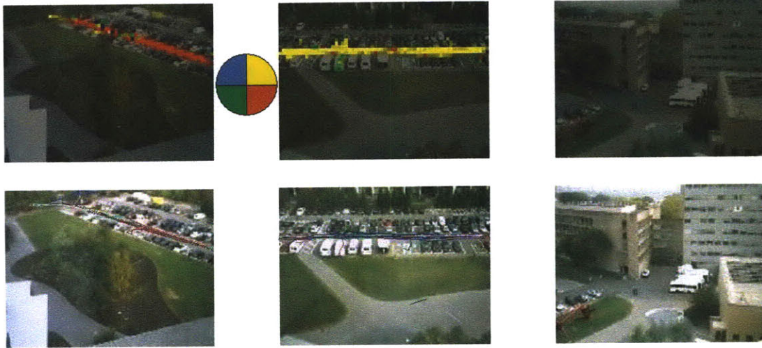
Figure 4-4: Learned cluster 1: the first row shows the learned activity cluster 1 and the second row shows the trajectories clustered into this activity. When visualizing activity clusters, moving directions are represented by different colors (red, yellow, blue and green), and the density of distributions over space and moving directions is proportional to the brightness of colors (high brightness means high density). When plotting trajectories, random colors are used to distinguish individual trajectories. This cluster represents vehicles entering the parking lot. These vehicles appear in Camera 1 and 2 , and may reappear in Camera 2 again later. However, they are not captured by Camera 3 because of the large gap between the views of Camera 2 and 3.
