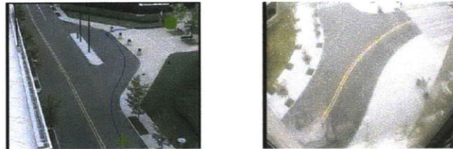
Figure 4-22: Abnormal activity 2: when a vehicle stopped and dropped off a person, the tracker didn't separate the person's trajectory from the vehicle's trajectory. Hence, it looked like a vehicle made an illegal right turn. In this case, it is the moving space which is unusual. The trajectory is plot in blue, and the starting and ending points of the trajectory are marked by green plus and dot.
