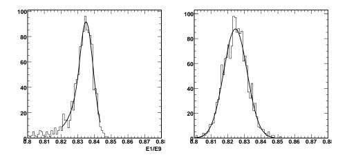
Figure 8. Distribution of the simulated E1/E9 ratio from the test beam data from 120 GeV electron (left) and with FastSim with the default setting of the Moliére radius (right).
