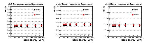
Figure 5. Mean fractional energy deposit in  $1 \times 1$  (E1),  $3 \times 3$  (E9) and  $5 \times 5$  (E25) crystal matrices in the test beam data and tuned GFLASH parameterization.
