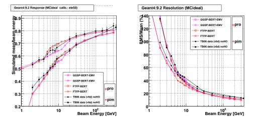
**Figure 2.** (Left) Mean energy responses of  $\pi^-$  (shown as circles) and protons (shown by squares) are compared with the predictions of QGSP\_BERT\_EMV physics list (shown by empty points) as a function of beam momentum. (Right) Energy resolutions for  $\pi^-$  and proton are compared with predictions of Full Simulation as a function of beam momentum.
