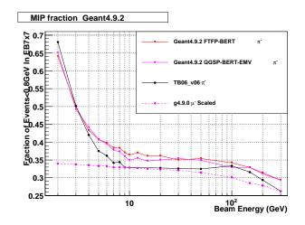
**Figure 4.** The fraction of  $\pi^-$ s with a MIP like signal in ECAL as a function of beam energy. Test beam results are compared with predictions of GEANT4 using the QGSP\_BERT and FTFP\_BERT physics lists.
