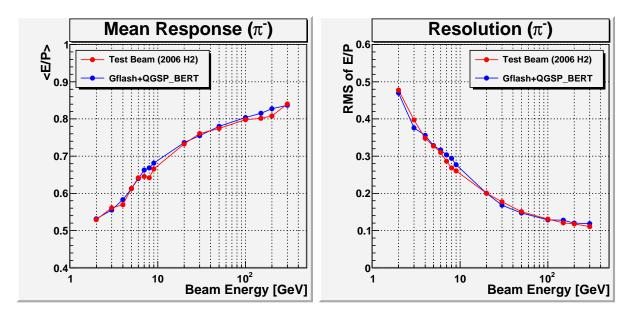
Figure 6. Mean energy response and energy resolution of  $\pi^-$  as a function of momentum from the test beam data and tuned GFLASH parameterization.
