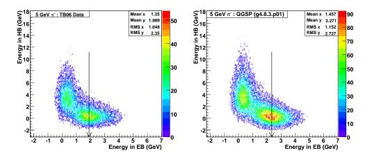
Figure 1. The measured energy in HCAL vs ECAL for 5 GeV  $\pi^-$  in the data (left), GEANT4 prediction (right) using the QGSP physics list. The simulated energy in ECAL is higher than what is observed for the test beam.
