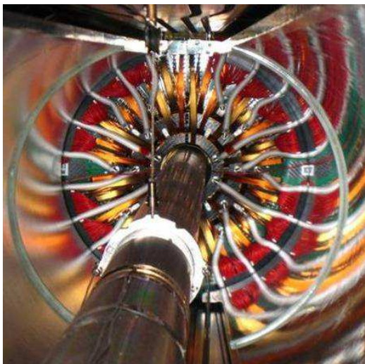
Figure 12. View of the barrel pixel detector in its final position inside CMS. On the left hand side, the central beam pipe and the detector end-flanges with cooling lines and power and signal cables can be seen. A picture of the connection area PP0 is shown on the right hand side.
