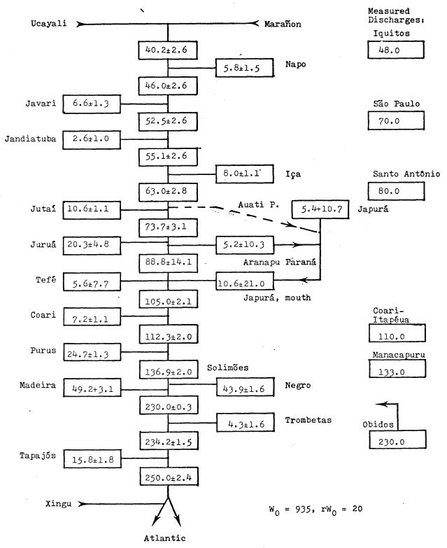
1977 Model Discharges (10<sup>3</sup> m<sup>3</sup>/sec) with the Aranapu Parana
