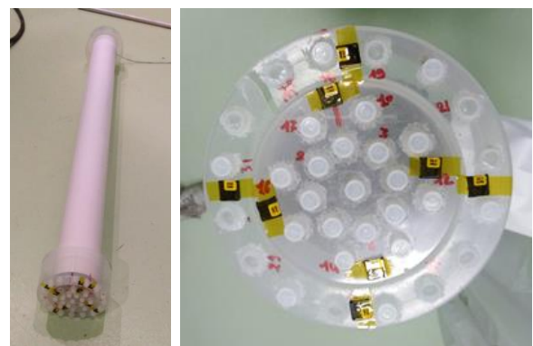
Fig. 3. Holding device for the detectors in the NB1 tangential channel.
