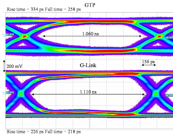
Figure 5. Eye diagram comparison between GLink and the GTP.
