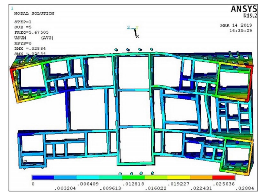
Figure 14. Five mode shapes resulting from free vibration analysis
