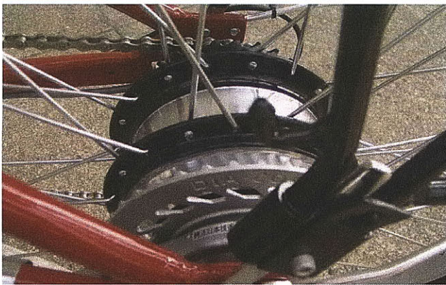
Fig. 3.2.1, hub motor that is used on an electric bicycle
