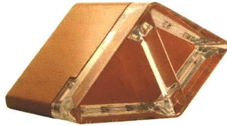
Fig. 5.1.2, RoboScooter G1 battery pack designed by MIT Smart Cities research group member Arthur Petron (left) and RoboScooter G1 battery pack, 36V 10AH (right)
