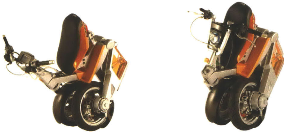
Fig. 6.1.4, the folding sequence of the RoboScooter
