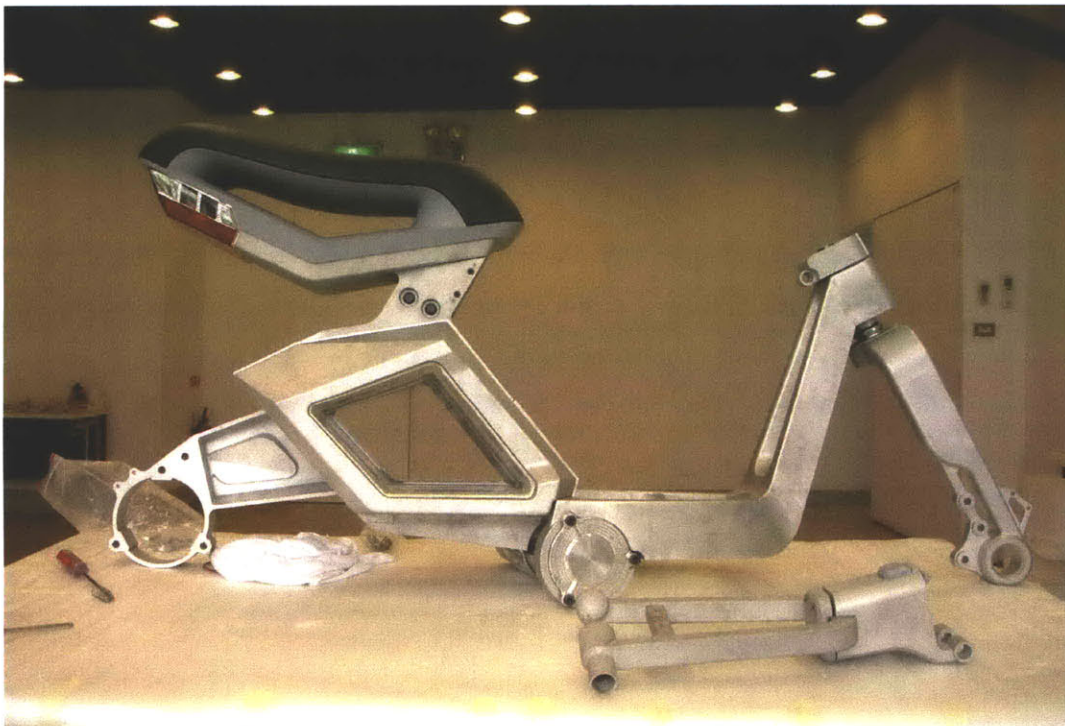
Fig. 4.2.8, the exposed aluminum frame of the RoboScooter G1
