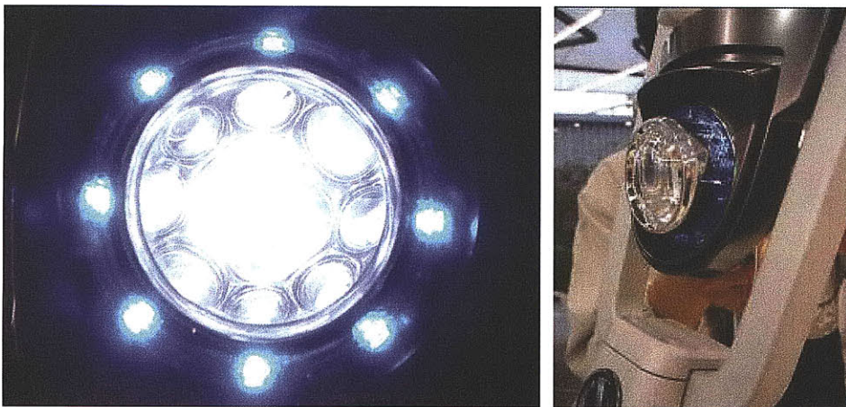
Fig. 4.5.4, the headlight is located in the front of the control console; it is powered by LED lights.
