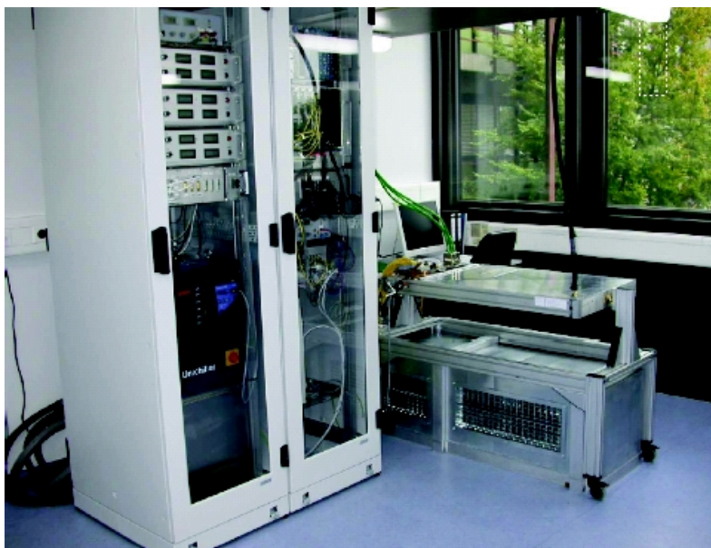
Figure 3: Photograph of the reception test setup in the clean room. The two racks in the foreground house all readout and service equipment, and a petal mounted in a rotating cradle can be seen in the background.
