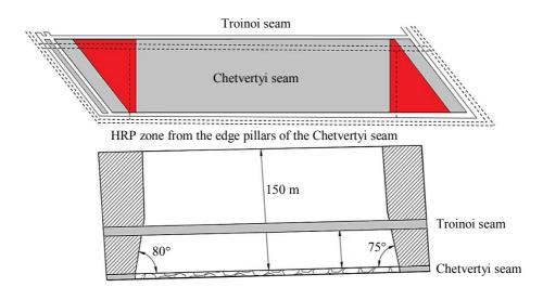
Fig.1. The current technological scheme with leaving the pillars in the edge parts of the extraction pillars
