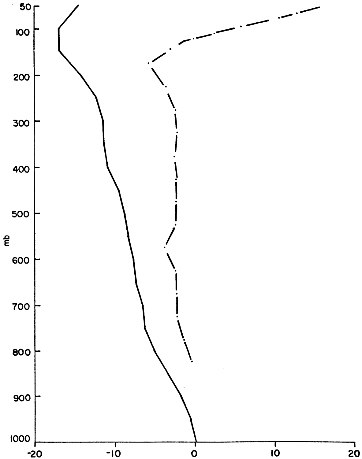
Figure 16. Distributions of vertical velocities ( 10^{-3} mb/s), calculated from the continuity equation (—) and the adiabatic thermodynamic equation (-·-·) for triangle EFC on August 28, 1973.
