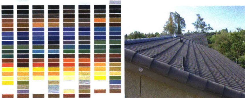
Figure 1-5: (left) A few of the “cool” color pigments analyzed by LBNL found in their online database. (right) A home with a colored cool tile roof installed. Source [55]
