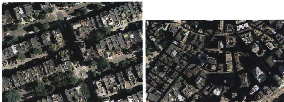
Figure 1-11: Black modified-bitumen roofs fill Boston's residential Back Bay (left) and commercial downtown areas (right), as is the case in many OECD cities. Source [8]
