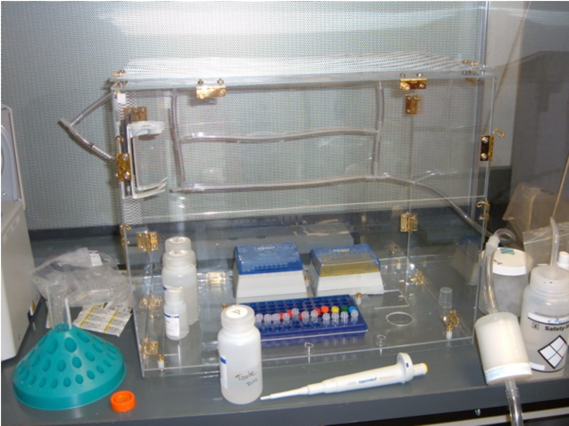
Figure 4.7: Plexiglas RNA extraction hood with quasi-laminar flow HEPA filtered air built by N. Levine and D. Levine.
