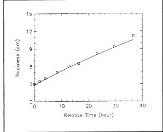
**Figure 3.** Saline ice thickness retrieval using polarimeteric time-series data. Squares represent the measured ice thickness. Solid curve indicates the evolution of reconstructed ice thickness using measured time-series data at 25 degree incident angle.
