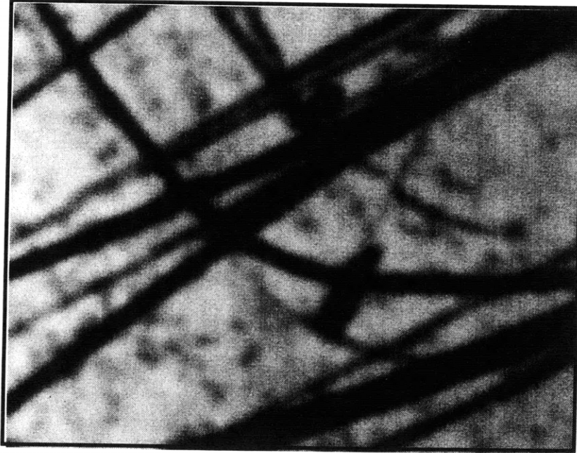
A cathodoluminescence micrograph from a 1 \mu\text{m} -thick ZnSe layer on a Zn-exposed, (2x4) reconstructed, 8 monolayer thick GaAs layer on a 4 \mu\text{m} graded InGaP layer. The surface was imaged at the ZnSe wavelength at a magnification of 1700x using a probe current of 32 nA and an acceleration voltage of 20 kV. The sample was grown in the Chemical Beam Epitaxy Laboratory which is under the direction of Professor Leslie A. Kolodziejski.
