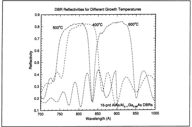
**Figure 2.** Reflectivities of 16 periods' AlAs/Al (0.11) Ga (0.89)As DBRs grown at temperatures ranging from 600 degrees C down to 400 degrees C. The shift in wavelength of the pass band is due to a calibration error and is not related to the growth temperature differences.
