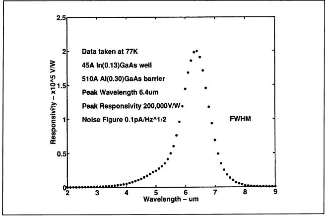
**Figure 5.** The normal incidence responsivity measured at 77K for a pseudomorphic InGaAs QWIP consisting of five periods of 4.5 nm of In<sub>0.13</sub>Ga<sub>0.87</sub>As and 51 nm of Al<sub>0.3</sub>Ga<sub>0.7</sub>As.
