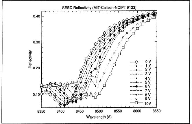
Figure 3. The measured reflectivity spectrum between 835 and 865 nm of a SEED modulator at selected voltages between 0 and 10 volts.
