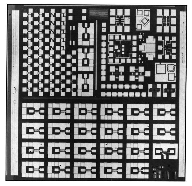
Photomicrograph of InAlAs/InGaAs High-Electron Mobility Transistor test chip fabricated at MIT.
